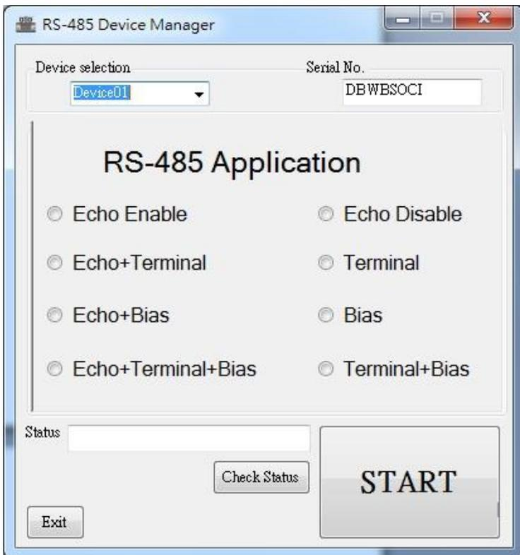
4. Operation for setting Device01: click 'Echo+Terminal' for the device's application setting and then click "START".
