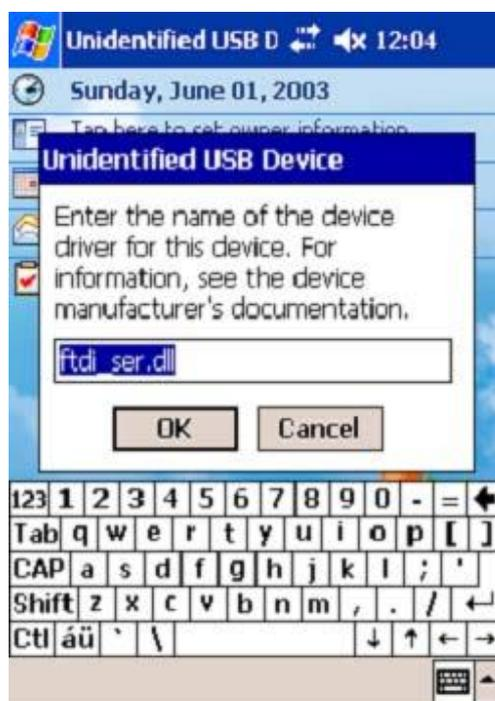
The device installation is now complete. The installation may be verified using the test program available from the Utilities page of the FTDI website.
