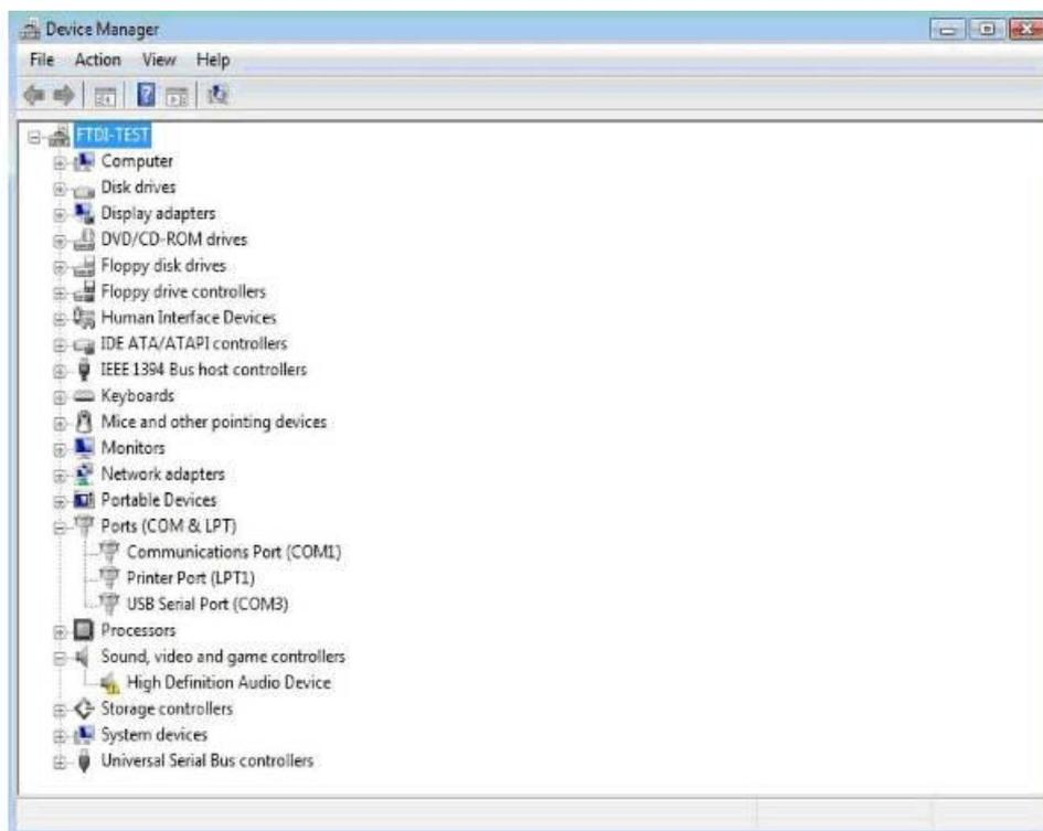
This screen shows the device connected to COM3.
