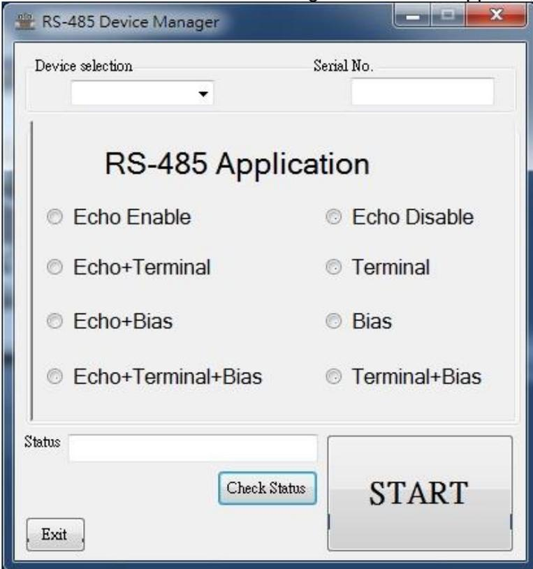
2. **RS-485 Device Manager** will detect all **UTS-485UI** devices connected to the PC, click **“Device selection”** drop down to select device.
