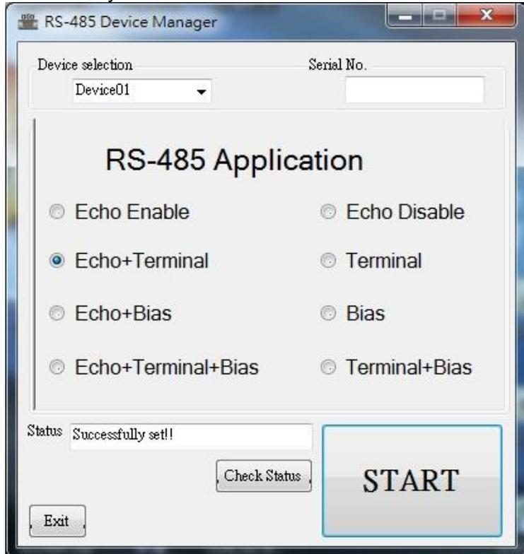
6. To confirm device's application setting, while UTS-485UI is still connected to the PC, Select device again then
