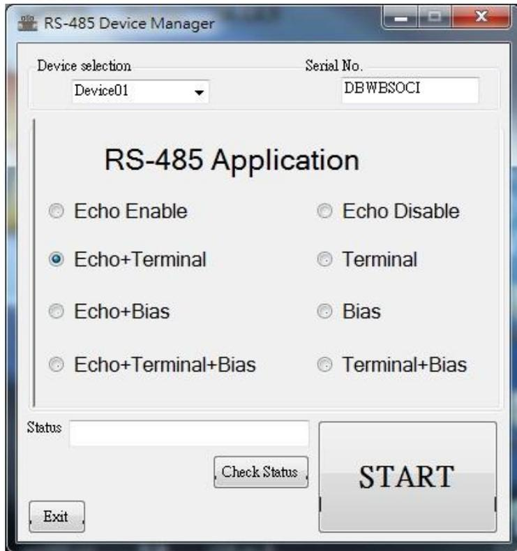
5. Wait until the block of the 'Serial No.' displays blank, and you have finished the device's application setting successfully.
